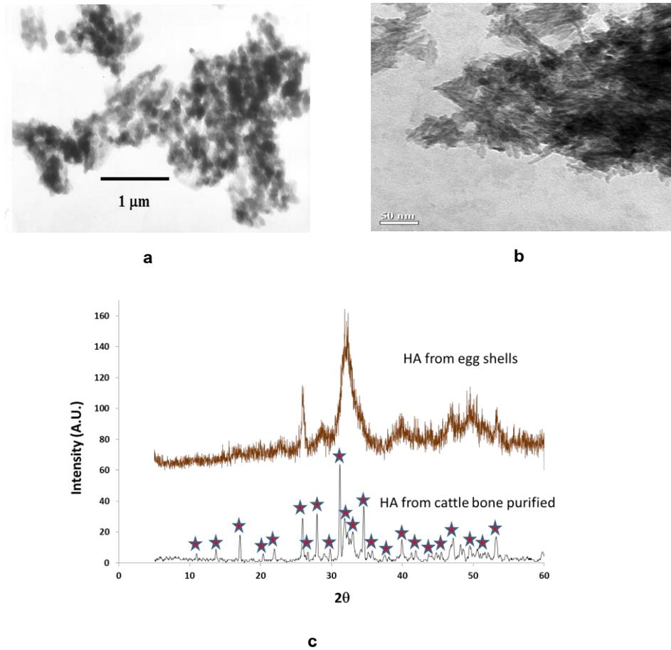
**Figure 2** Nanosized HA was synthesized from a) cattle bones and b) egg shells and c) XRD patterns displayed the pure phase in both types of HA
