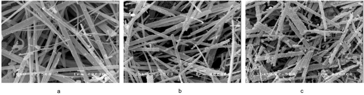
**Figure 5** Hydroxyapatite whisker from purified cattle bone were prepared at 150°C for a) 6 h b) 12 h and c) 24 h in autoclave reactor
